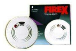
This Stand Alone Smoke Detector is available with dual ionization smoke sensing chamber. Stand Alone Smoke Detector is fast and easy to install and is mounted on a bracket which needs no wiring and it runs on a 9V DC battery. The horn output is 85 decibels at 10 ft. These smoke alarms should be placed in family households, in each individual unit of multiple-family buildings, schools, colleges, homes, offices, factories and just anywhere.
