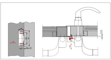
PHA 2421 adjustable latch keeper for aluminium narrow-stile doors
